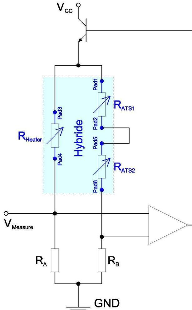
Figure 3: Outline of a measurement electronics using a Wheatstone-bridge.
