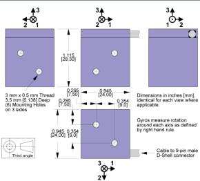
I wo 3 mm x 0.5 mm threaded holes are provided on each of three orthogonal faces for mounting
