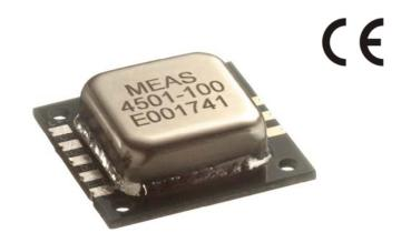
The Model 4503 is an economical board mountable accelerometer with micro-g resolution. The output is signal conditioned and temperature compensated and offers an optional 2.5V reference for single-ended or differential output measurements. The model 4503 is available in ranges from ±2g to ±200g with a frequency response up to 1500Hz. The gas damped MEMS sensing element provides stable long-term performance.
