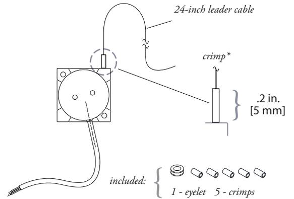
\*note: crimped stop prevents leader cable from retracting into sensor body
