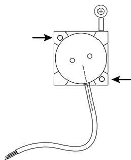
\*-includes: 4) #2-56 x 3/8" pan head mounting screws with washers
