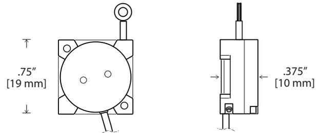
Introducing the world's smallest stringpot. The M150 is smaller than a thumbprint and occupies a tiny space of only .74 x .74 x .38 inches. With a full stroke measurement range of 1.5 inches, the M150 has been designed for many aerospace and automotive space-critical test applications such as throttle position and crash-test instrumentation.
